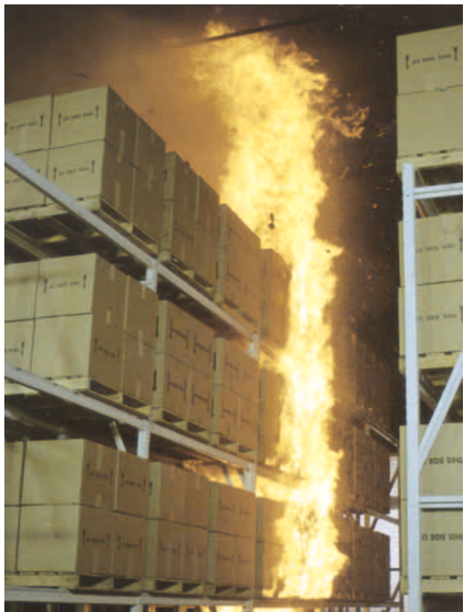
Rack storage fire test of cartoned commodities
